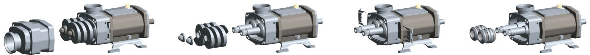
1. Removal of pump casing and cover
